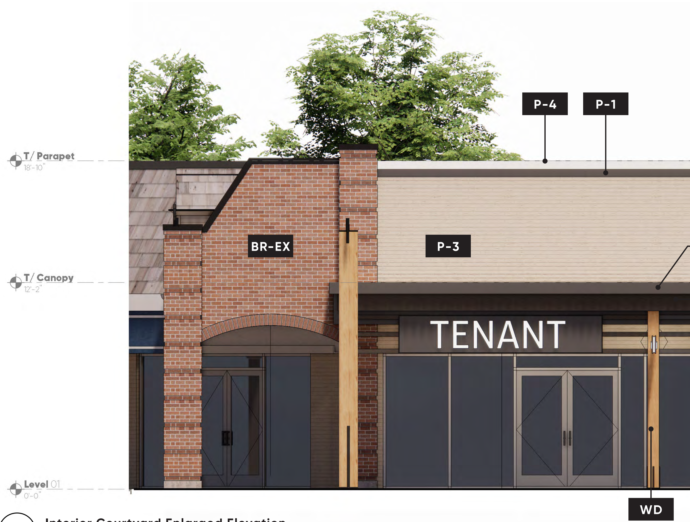
01 Interior Courtyard Enlarged Elevation Scale: 3/8" = 1'-0"
