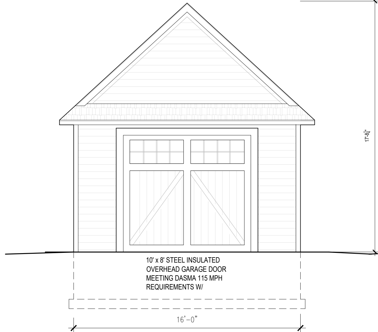
1 NORTH (FRONT) ELEVATION SCALE 1/4" = 1'-0"
