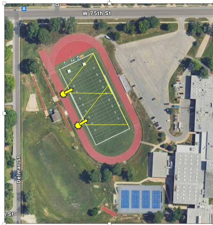
Sample Temporary Lighting Orientation with 2 lights
