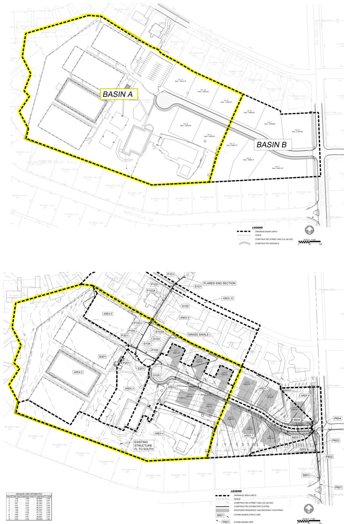
Figure 2 – Drainage Basins from the November 2016 Drainage Study
