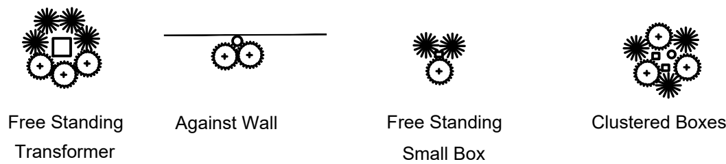
TYPICAL UTILITY BOX SCREENING DETAILS - NTS
