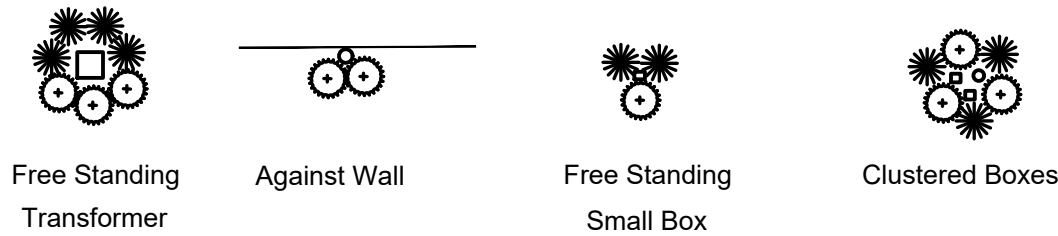
TYPICAL UTILITY BOX SCREENING DETAILS - NTS
